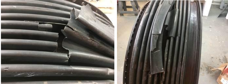
Fig 19. Ruptured bellows Feb 2017
